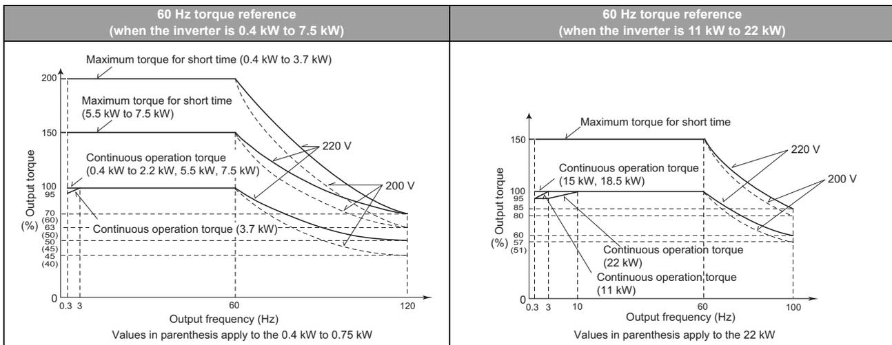
The maximum short-time torque indicates the maximum torque characteristics within 60 s. For the motor constant under Real sensorless vector control, please contact your sales representative.
