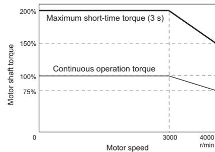
When the input voltage is low, the torque may be reduced.
